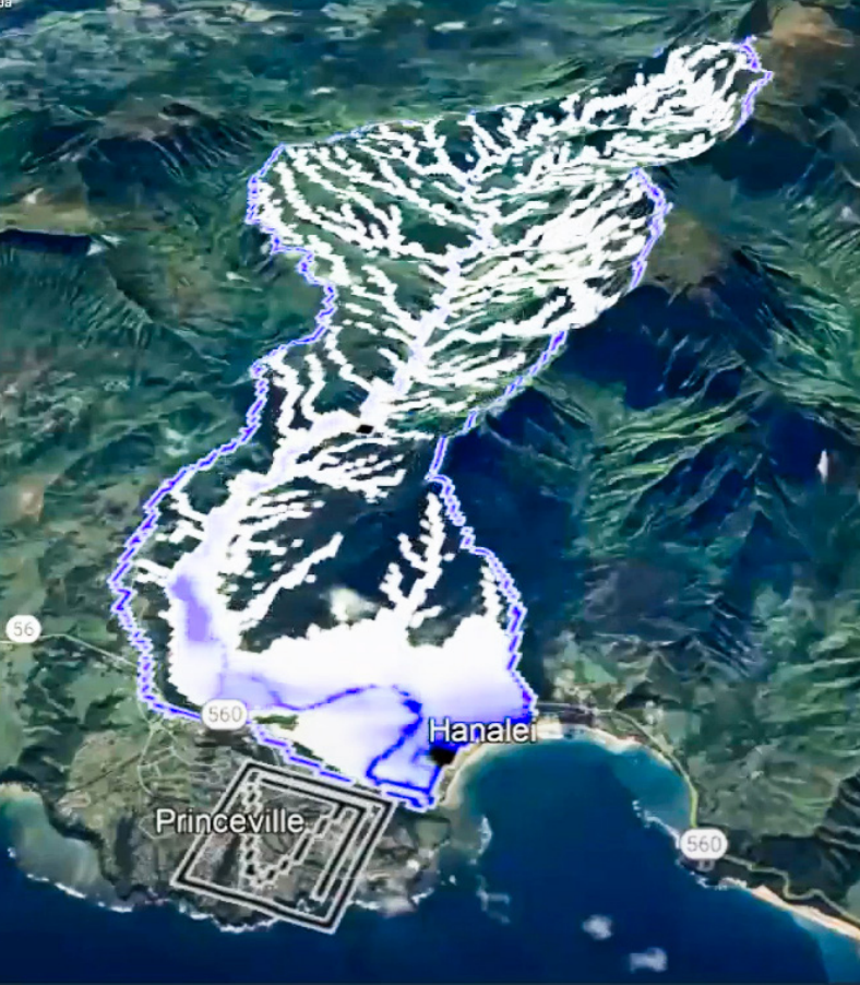
Figure 4: Screenshot from a preliminary 2D flood model simulation of the Hanalei watershed in North Kaua'i produced with the GSSHA model. (Credit: Brian Gorberg)
